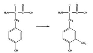
Figure 1. Tyrosine treated with nitric acid produces yellow xanthoproteic acid.
